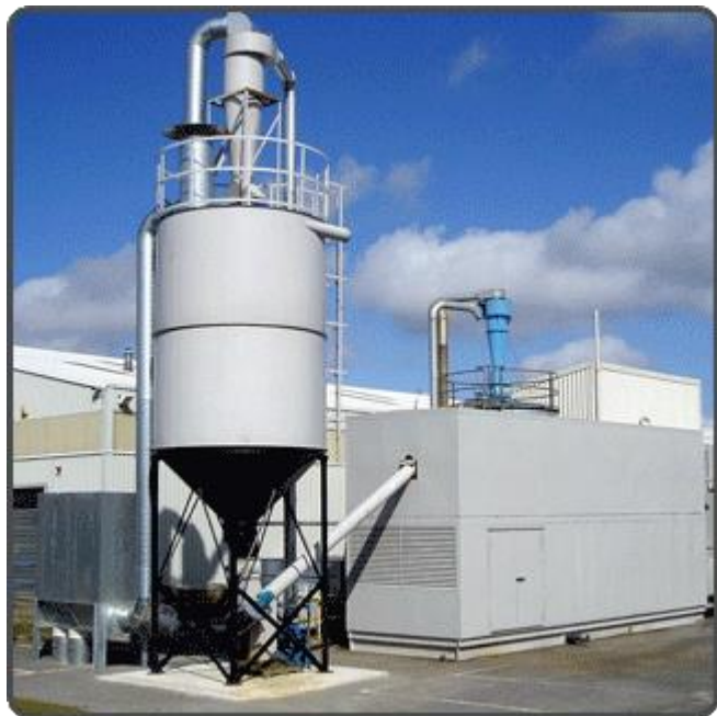
250kWe Wood Gasification System, Photo Courtesy of Sustainable Energy Ltd
